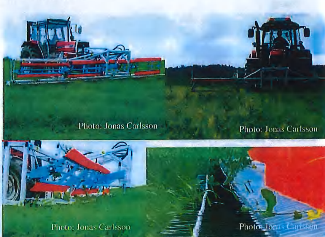
Fig. 7. Weed mower CombCut (upper left and right). Close up pictures of the brush reel (lower left) and the knives (lower right). Photo: Jonas Carlsson, JustCommonSense AB.
