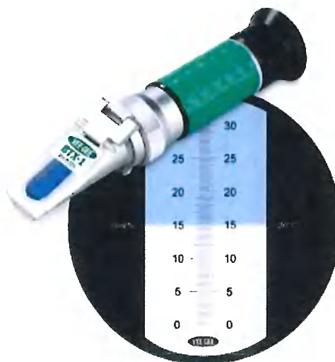
A refractometer and the Brix reading scale. Photo via: highbrixgardens.com
