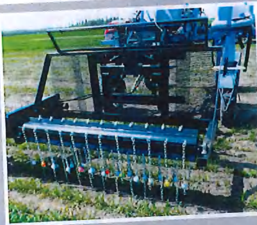
Hail Simulator mounted on SARDA's spider sprayer.
