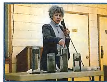
Yamily demonstrating a visual soil aggregate stability test
