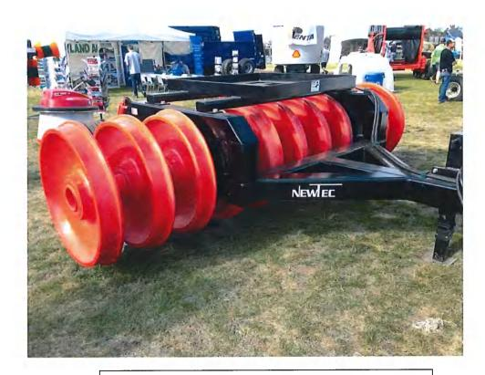
Silage packer made out of recycled Rail car wheels.
