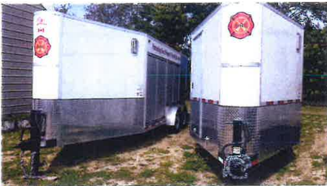
14' "V Nose," Twin 7,000 lb. Axles, 4 Roll-Up Doors, 8 Slide-Out Trays, 12K Pop-Up Jack
