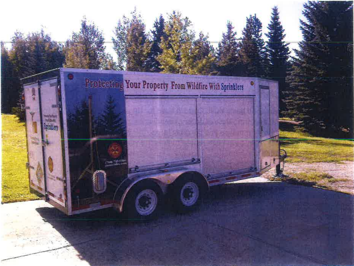
14' "V Nose," Twin 7,000 lb. Axles, 4 Roll-Up Doors, 8 Slide-Out Trays, 12K Pop-Up Jack
